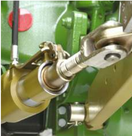
Hydraulically controlled lateral stabiliser HGST
